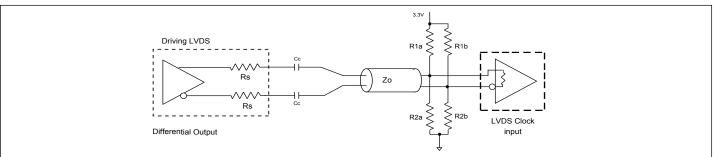
Figure 3. Differential Output Driving LVDS
