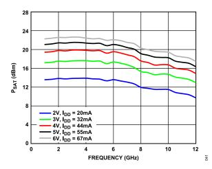
Figure 41.  $P_{SAT}$  vs. Frequency, 1 GHz to 12 GHz, for Various Supply Voltages and  $I_{DD}$ ,  $R_{BIAS}$  = 1.1 k $\Omega$
