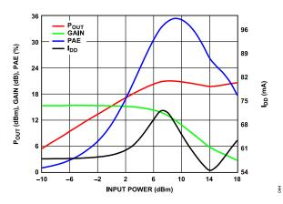
Figure 44.  $P_{OUT}$ , Gain, PAE, and  $I_{DD}$  vs. Input Power, Power Compression at 1 GHz,  $V_{DD}$  = 5 V,  $I_{DQ}$  = 55 mA
