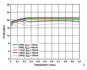
Figure 33. P1dB vs. Frequency, 0.01 GHz to 1.0 GHz, for Various Bias Resistor Values and I<sub>DQ</sub>, V<sub>DD</sub> = 5 V
