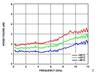
Figure 28. Noise Figure vs. Frequency, 200 MHz to 12 GHz, for Various Temperatures,  $V_{DD}$  = 5 V,  $I_{DO}$  = 55 mA
