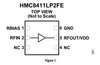
The HMC8411LP2FE also features inputs and outputs that are internally matched to 50  $\Omega$ , making the device ideal for surface-mounted technology (SMT)-based, high capacity microwave radio applications.
