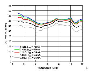
Figure 65. OIP2 vs. Frequency, 1 GHz to 12 GHz, for Various Bias Resistor Values and  $I_{DQ}$ ,  $V_{DD}$  = 5 V
