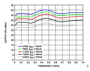
Figure 62. OIP2 vs. Frequency, 0.01 GHz to 1.0 GHz, for Various Bias Resistor Values and  $I_{DQ}$ ,  $V_{DD}$  = 5 V
