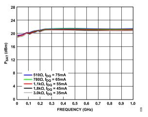
Figure 39.  $P_{SAT}$  vs. Frequency, 0.01 GHz to 1.0 GHz, for Various Bias Resistor Values and  $I_{DQ}$ ,  $V_{DD}$  = 5 V
