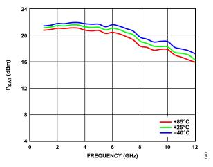
Figure 40.  $P_{SAT}$  vs. Frequency, 1 GHz to 12 GHz, for Various Temperatures,  $V_{DD}$  = 5 V,  $I_{DQ}$  = 55 mA
