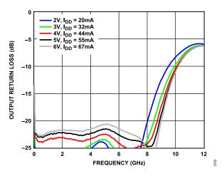
Figure 19. Output Return Loss vs. Frequency for Various Supply Voltages and  $I_{DD}$ ,  $R_{BIAS} = 1.1 k\Omega$
