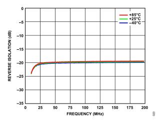
Figure 20. Reverse Isolation vs. Frequency, 10 MHz to 200 MHz, for Various Temperatures,  $V_{DD}$  = 5 V,  $I_{DQ}$  = 55 mA
