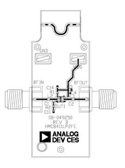
Figure 71. EV1HMC8411LP2F Printed Circuit Board (PCB)
