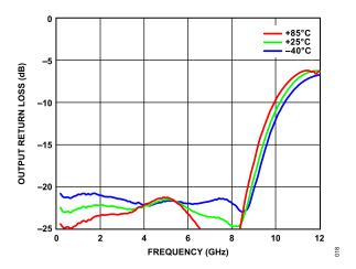
Figure 18. Output Return Loss vs. Frequency, 200 MHz to 12 GHz, for Various Temperatures,  $V_{DD}$  = 5 V,  $I_{DO}$  = 55 mA
