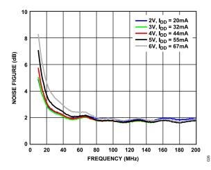
Figure 26. Noise Figure vs. Frequency, 10 MHz to 200 MHz, for Various Supply Voltages and  $I_{DD}$ ,  $R_{BIAS} = 1.1 \text{ k}\Omega$
