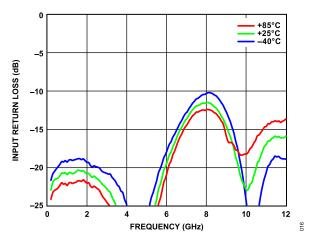
Figure 16. Input Return Loss vs. Frequency, 200 MHz to 12 GHz, for Various Temperatures,  $V_{DD}$  = 5 V,  $I_{DQ}$  = 55 mA
