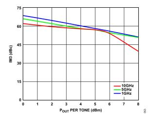
Figure 53. IM3 vs.  $P_{OUT}$  per Tone for Various Frequencies,  $V_{DD}$  = 5 V,  $I_{DQ}$  = 55 mA
