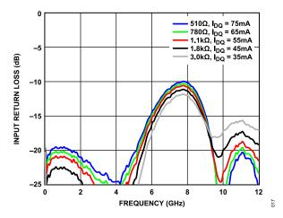
Figure 17. Input Return Loss vs. Frequency for Various Bias Resistor Values and  $I_{DQ}$ ,  $V_{DD}$  = 5 V
