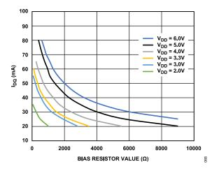
Figure 68.  $I_{DQ}\,vs.$  Bias Resistor Value and at Various  $V_{DD}$  Values
