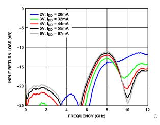
Figure 14. Input Return Loss vs. Frequency for Various Supply Voltages and  $I_{DD}$ ,  $R_{BIAS}$  = 1.1 k $\Omega$
