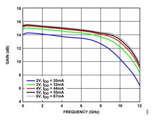
Figure 9. Gain vs. Frequency for Various Supply Voltages and Currents ( $I_{DD}$ ),  $R_{BIAS} = 1.1 \ k\Omega$
