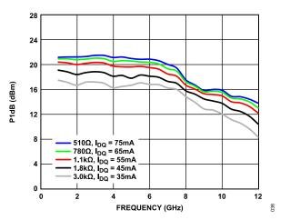
Figure 36. P1dB vs. Frequency, 1 GHz to 12 GHz, for Various Bias Resistor Values and  $I_{DQ}$ ,  $V_{DD}$  = 5 V
