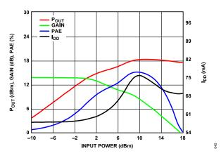
Figure 45.  $P_{OUT}$ , Gain, PAE, and  $I_{DD}$  vs. Input Power, Power Compression at 10 GHz,  $V_{DD}$  = 5 V,  $I_{DO}$  = 55 mA
