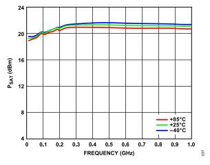
Figure 37.  $P_{SAT}$  vs. Frequency, 0.01 GHz to 1.0 GHz, for Various Temperatures,  $V_{DD}$  = 5 V,  $I_{DQ}$  = 55 mA
