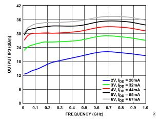
Figure 55. OIP3 vs. Frequency, 0.01 GHz to 1.0 GHz, for Various Supply Voltages and I<sub>DD</sub>,  $R_{BIAS}$  = 1.1 k $\Omega$
