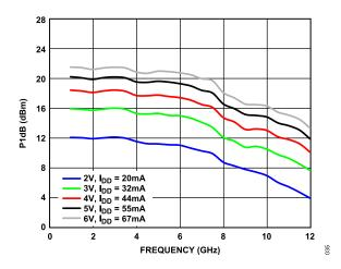
Figure 35. P1dB vs. Frequency, 1 GHz to 12 GHz, for Various Supply Voltages and  $I_{DD}$ ,  $R_{BIAS}$  = 1.1 k $\Omega$
