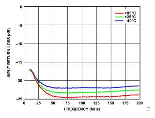
Figure 13. Input Return Loss vs. Frequency, 10 MHz to 200 MHz, for Various Temperatures,  $V_{DD}$  = 5 V,  $I_{DO}$  = 55 mA
