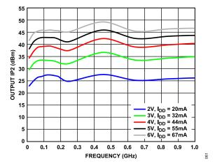
Figure 61. OIP2 vs. Frequency, 0.01 GHz to 1.0 GHz, for Various Supply Voltages and I<sub>DD</sub>,  $R_{BIAS}$  = 1.1 k $\Omega$
