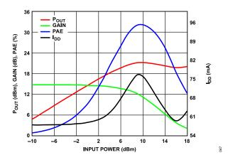
Figure 47.  $P_{OUT}$ , Gain, PAE, and  $I_{DD}$  vs. Input Power, Power Compression at 5 GHz,  $V_{DD}$  = 5 V,  $I_{DQ}$  = 55 mA
