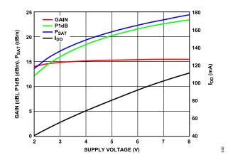
Figure 48. P1dB, Gain, PAE, and I\_{DD} vs. Supply Voltage, Power Compression at 1 GHz,  $R_{BIAS}$  = 1.1 k $\Omega$
