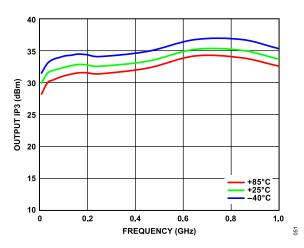
Figure 51. OIP3 vs. Frequency, 0.01 GHz to 1.0 GHz, for Various Temperatures,  $V_{DD}$  = 5 V,  $I_{DQ}$  = 55 mA
