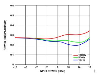
Figure 50. Power Dissipation vs. Input Power at  $T_A = 85^{\circ}$ C,  $V_{DD} = 5 V$ ,  $I_{DQ} = 55 mA$
