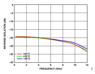
Figure 23. Reverse Isolation vs. Frequency, 200 MHz to 12 GHz, for Various Temperatures,  $V_{DD}$  = 5 V,  $I_{DQ}$  = 55 mA
