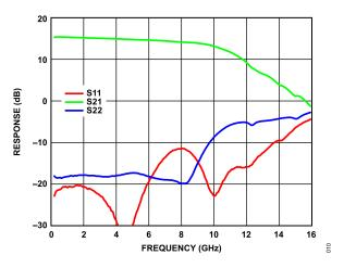
Figure 10. Broadband Gain and Return Loss (Response) vs. Frequency, 200 MHz to 16 GHz, V<sub>DD</sub> = 5 V, I<sub>DQ</sub> = 55 mA
