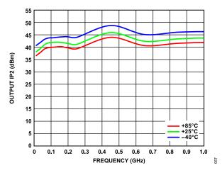
Figure 57. OIP2 vs. Frequency, 0.01 GHz to 1.0 GHz, for Various Temperatures,  $V_{DD}$  = 5 V,  $I_{DQ}$  = 55 mA
