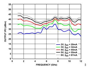
Figure 64. OIP2 vs. Frequency, 1 GHz to 12 GHz, for Various Supply Voltages and  $I_{DD}$ ,  $R_{BIAS}$  = 1.1 k $\Omega$
