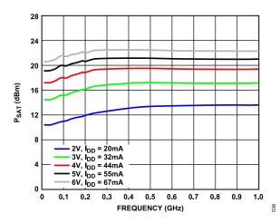
Figure 38.  $P_{SAT}$  vs. Frequency, 0.01 GHz to 1.0 GHz, for Various Supply Voltages and  $I_{DD}$ ,  $R_{BIAS} = 1.1 \text{ k}\Omega$
