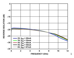
Figure 21. Reverse Isolation vs. Frequency for Various Supply Voltages and  $I_{DD},\,R_{BIAS}$  = 1.1 k $\Omega$
