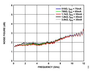
Figure 30. Noise Figure vs. Frequency, 200 MHz to 12 GHz, for Various Bias Resistor Values and  $I_{DQ},\,V_{DD}$  = 5 V
