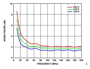
Figure 25. Noise Figure vs. Frequency, 10 MHz to 200 MHz, for Various Temperatures,  $V_{DD}$  = 5 V,  $I_{DO}$  = 55 mA
