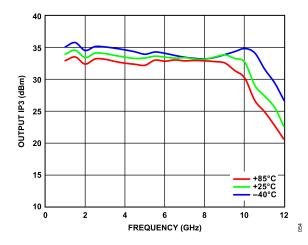
Figure 54. OIP3 vs. Frequency, 1 GHz to 12 GHz, for Various Temperatures,  $V_{DD}$  = 5 V,  $I_{DQ}$  = 55 mA
