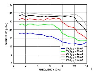
Figure 58. OIP3 vs. Frequency, 1 GHz to 12 GHz, for Various Supply Voltages and  $I_{DD}$ ,  $R_{BIAS}$  = 1.1 k $\Omega$
