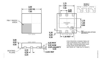
Figure 73. 6-Lead Lead Frame Chip Scale Package [LFCSP] 2 mm × 2 mm Body and 0.85 mm Package Height (CP-6-12) Dimensions shown in millimeters
