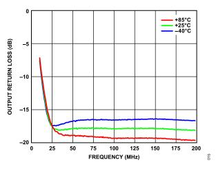
Figure 15. Output Return Loss vs. Frequency, 10 MHz to 200 MHz, for Various Temperatures, V<sub>DD</sub> = 5 V, I<sub>DO</sub> = 55 mA
