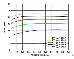
Figure 32. P1dB vs. Frequency, 0.01 GHz to 1.0 GHz, for Various Supply Voltages and  $I_{DD}$ ,  $R_{BIAS}$  = 1.1 k $\Omega$
