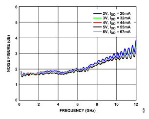
Figure 29. Noise Figure vs. Frequency, 200 MHz to 12 GHz, for Various Supply Voltages and I<sub>DD</sub>,  $R_{BIAS}$  = 1.1 k $\Omega$
