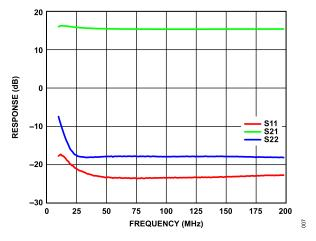
Figure 7. Gain and Return Loss (Response) vs. Frequency, 10 MHz to 200 MHz,  $V_{DD}$  = 5 V,  $I_{DO}$  = 55 mA
