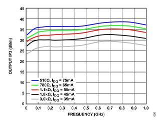
Figure 56. OIP3 vs. Frequency, 0.01 GHz to 1.0 GHz, for Various Bias Resistor Values and  $I_{DQ}$ ,  $V_{DD}$  = 5 V
