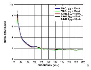
Figure 27. Noise Figure vs. Frequency, 10 MHz to 200 MHz, for Various Bias Resistor Values and  $I_{DO}$ ,  $V_{DD}$  = 5 V
