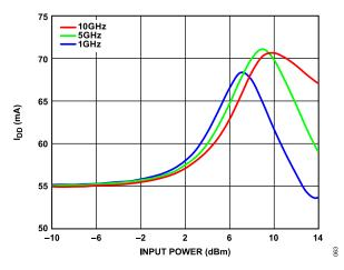
Figure 63.  $I_{DD}$  vs. Input Power for Various Frequencies,  $V_{DD}$  = 5 V
