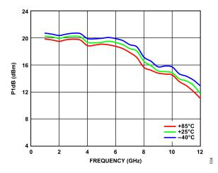
Figure 34. P1dB vs. Frequency, 1 GHz to 12 GHz, for Various Temperatures,  $V_{DD}$  = 5 V,  $I_{DQ}$  = 55 mA
