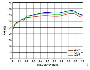
Figure 43. PAE vs. Frequency, 0.01 GHz to 1.0 GHz, for Various Temperatures,  $V_{DD}$  = 5 V,  $I_{DQ}$  = 55 mA
