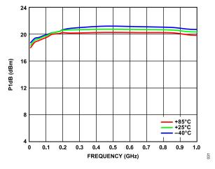
Figure 31. P1dB vs. Frequency, 0.01 GHz to 1.0 GHz, for Various Temperatures, V<sub>DD</sub> = 5 V, I<sub>DQ</sub> = 55 mA
