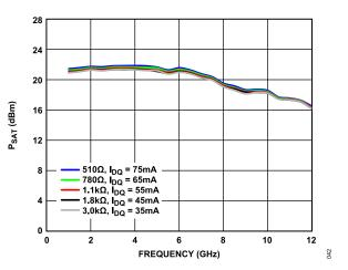
Figure 42.  $P_{SAT}$  vs. Frequency, 1 GHz to 12 GHz, for Various Bias Resistor Values and  $I_{DQ}$ ,  $V_{DD}$  = 5 V
