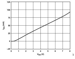
Figure 67.  $I_{DQ}$  vs.  $V_{DD}$ , Representative of a Typical Device,  $R_{BIAS}$  = 1.1 k $\Omega$
