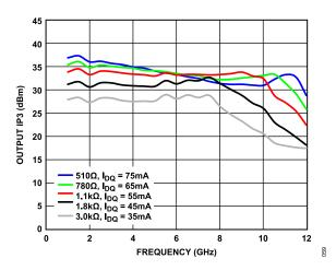
Figure 59. OIP3 vs. Frequency, 1 GHz to 12 GHz, for Various Bias Resistor Values and  $I_{DQ}$ ,  $V_{DD}$  = 5 V
