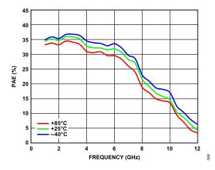
Figure 46. PAE vs. Frequency, 1 GHz to 12 GHz, for Various Temperatures, V<sub>DD</sub> = 5 V, I<sub>DQ</sub> = 55 mA
