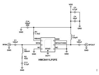
Figure 72. EV1HMC8411LP2F Evaluation Board Schematic
