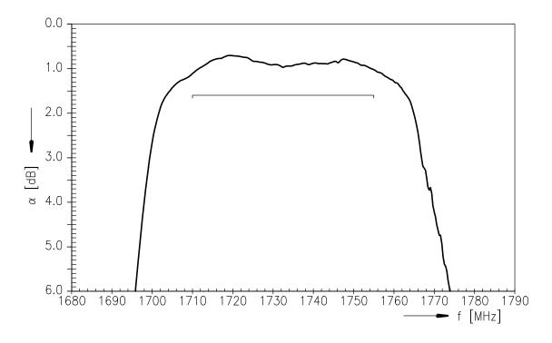
SAW ComponentsB8333SAW Tx Filter1732.5 MHz
