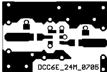
Figure 4: Optimised PCB layout for SAW filters in DCC6E package, pinning 2,4 (top side, scale 1:1).
