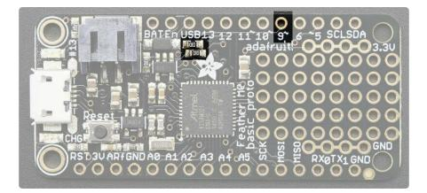
In Arduino, you can read this pin's voltage, then double it, to get the battery voltage.
