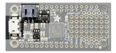
The above shows the Micro USB jack (left), LiPoly JST jack (top left), as well as the 3.3V regulator and changeover diode (just to the right of the JST jack) and the LiPoly charging circuitry (to the right of the Reset button).
