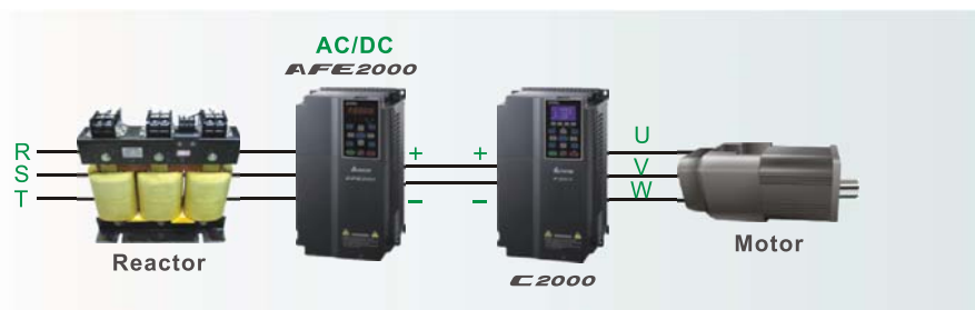
This figure is for demonstration purposes only, please refer to standard wiring diagrams for wiring details.
