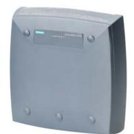
IWLAN access point, SCALANCE W786-2 RJ45, 2 radios, 6 R-SMA antenna connections, IEEE 802.11a/b/g/h/n, 2.4/5 GHz, gross 450 Mbit/s per radio, 1 x RJ45 (max. 1 Gbit/s), PoE, 24 V DC, IP65, (-40 to +60 °C), WPA2/802.111/e, Observe national approval! (Cert. ID: EAPN-W2-RJ-E3) Includes MPCIE-R1-ABGN-U3 Scope of delivery: Manuals on CD, de/en 1 x terminal block, only for operation in Israel.
