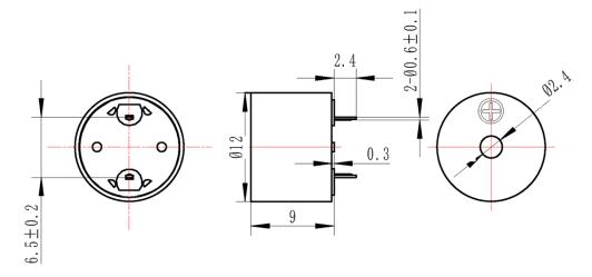
General tolerance =  $\pm 0.5$  mm and all measurements in mm unless otherwise noted.
