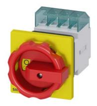
SENTRON, Switch disconnector 3LD, emergency switching-off switch, 4-pole, lu: 16 A, operating power / at AC-23 A 400 V: 7.5 kW, front-mounted, rotary operating mechanism, Red / yellow, central mounting 22.5 mm of the handle
