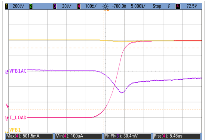
VCC1 = 3.8 V Vout = 1.2 V PWM Mode Figure 7-3. VDD1 Rising Load Transient Response
