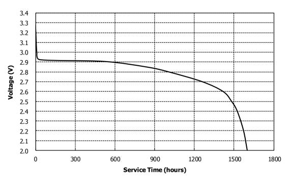
Discharge method:15K $\Omega$ , 24 hours/day EV 2.0V temperature of 20±2°C
