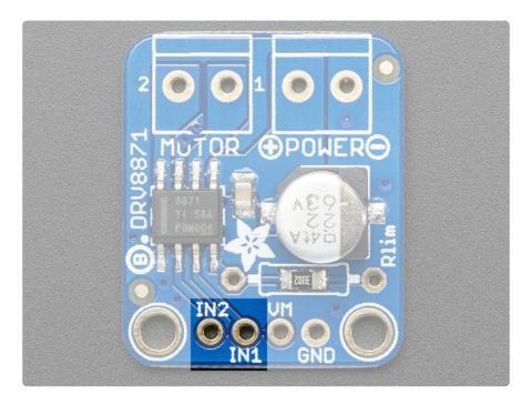
These are the inputs to the motor control. IN2 goes to OUT2, IN1 goes to OUT1. Use up to 5.5V DC logic on these pins. You can PWM the inputs up to 200KHz, but lower frequencies will be more efficient.
