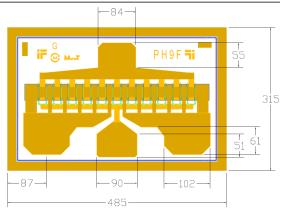
Chip Dimensions: 485 x 315 microns Chip Thickness: 100 microns
