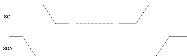
Figure 33: I 2 C START and STOP Conditions
