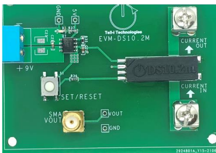
Figure 4. Regular Probing Location and Polarity
