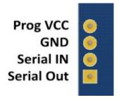
Note: Serial connection is 3.3V TTL. The MReX-PROG USB to serial adaptor can be provided for serial interfacing.
