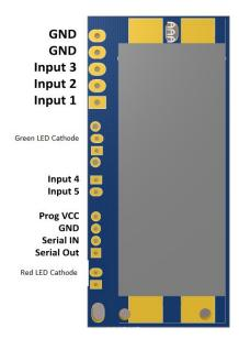
Only the Cathode connections of the LEDS are shown here. They are connected to an open drain output. As shown in the simplified schematic above, it is the users responsibility to select a resistor that suits the application, and then connect to a suitable power source that has a common GND.
