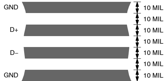
Figure 18. Arrangement of Signal Tracks
