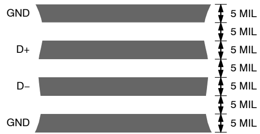
Figure 28. Arrangement of Signal Tracks
