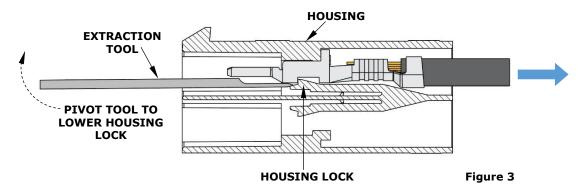
**CAUTION:** This extraction tool should be used to extract the terminal only. Using it for unintended purposes may cause injury or damage to parts. Be careful not to deform the end of the terminal.
