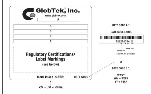
A=DC/DC Switching Power Supply B=P/N: (料号) GTDJ1000USB-F(R6B) C=Model (型号) GTD83050-0505 D=Input (输入)12-24 Vdc, 1A max E=Output (输出)5.0 V === 1.0 A, 5.0W
