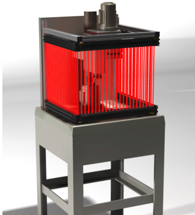
Figure 48. Cascaded light screens guarding a u-shaped cell
