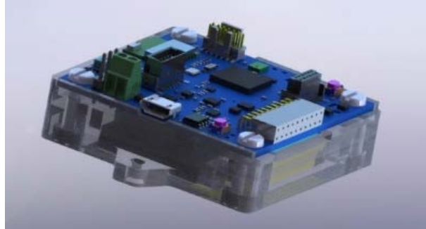
Figure 30. Core system board fastened with bolts
