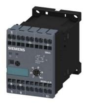
Timing relay, electronic ansprechverzögert 1 change-over contact 24 V AC/DC, 200 to 240 V AC at 50/60 Hz AC 0.05 s to 100 h Overall width 45 mm Spring-type terminal
