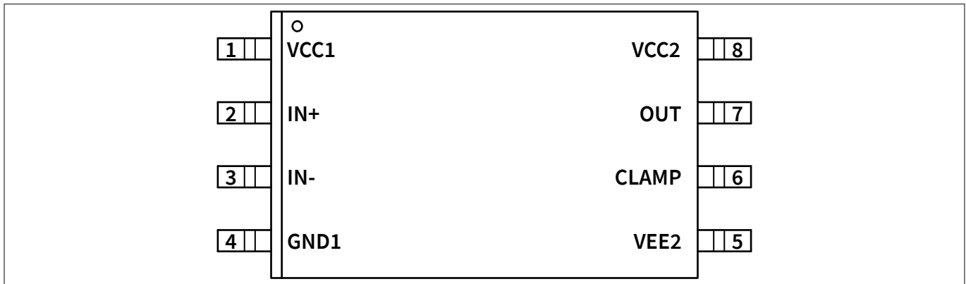
Figure 5 PG-DSO-8 (top view)
