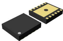
DFN(PLP)2730-12 2.7 mm x 3.0 mm x 0.6 mm
