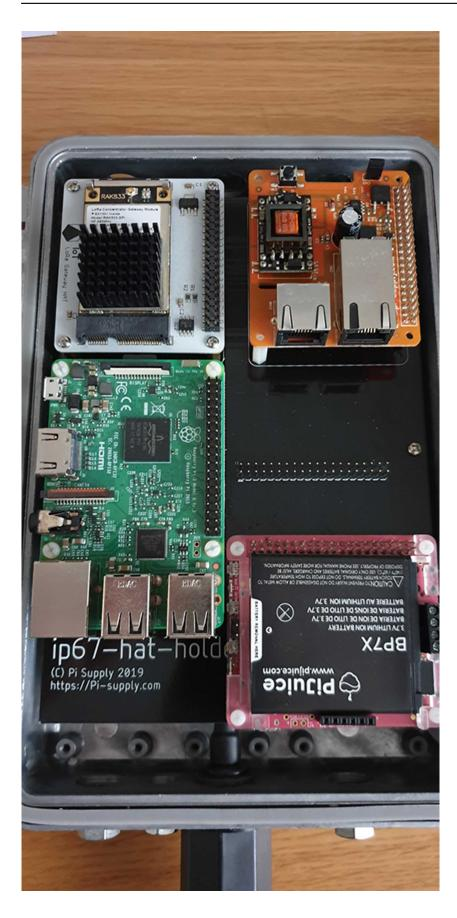
**Step 5** - Now you can add any cables that need connecting such as the PoE ethernet cables and the LoRa Gateway antenna cables too. Also it is important that you connect the ribbon cable from the Raspberry Pi GPIO header to the GPIO header on the HAT holder.
