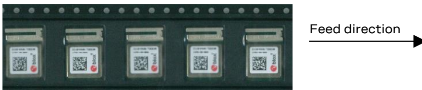
Figure 11: Orientation of NINA-W132 module on tape
