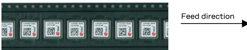
Figure 10: Orientation of NINA-W131 module on tape
