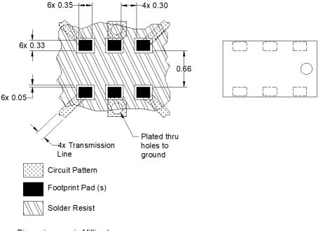
Dimensions are in Millimeters Mounting Footprint
