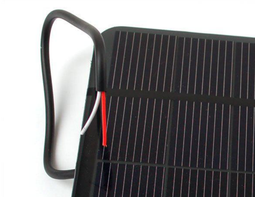
Strip and tin the inner wires.
