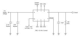
TV Series Clipped Sinewave Test Circuit
