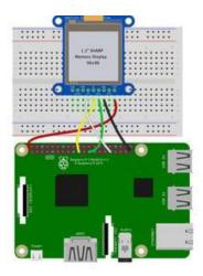
Raspberry Pi GND to LCD Gnd Raspberry Pi 3.3V to LCD Vin Raspberry Pi SCK (GPIO 11) to LCD Clk Raspberry Pi MOSI (GPIO 10) to LCD DI Raspberry Pi GPIO 6 to LCD CS
