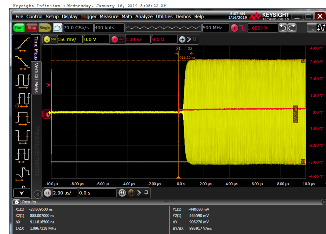
Figure 25. 6dB Gain Reduction Transient Time
