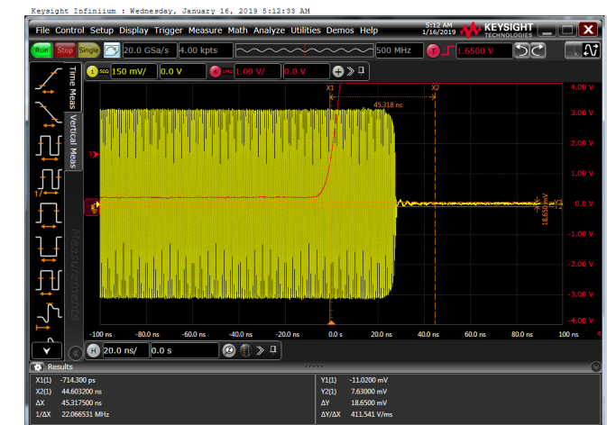
Figure 26. 6dB Gain Increase Transient Time
