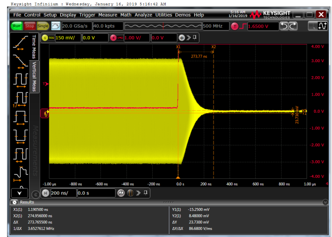
Figure 24. RX Mode to Standby Transient Time
