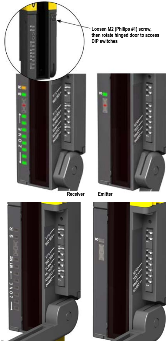
Figure 41. Accessing the configuration switches
