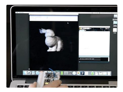
Also notice in the upper right corner of the dialog box at the top that the calibration of each sensor is displayed. It's important to calibrate the BNO055 sensor so that the most accurate readings are retrieved. Each sensor on the board has a separate calibration status from 0 (uncalibrated) up to 3 (fully calibrated). Check out the <a href="video">video</a> and information from this guide for how to best calibrate the BNO055 sensor (https://adafru.it/kA1).
