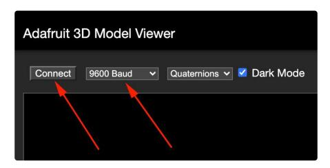
When the security window pops up, pick the matching Serial/COM port for your board running the AHRS sketches. Make sure the serial port isn't open in Arduino or something else.
