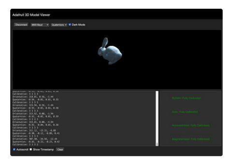
That raw data is all fine and good, but we want to see what they mean in 3D space, right? Traditionally, a Processing sketch would be used to read the serial data and convert it to a 3D rotation - but thanks to Web Serial API we can use any Chrome browser - a lot easier than installing Processing! (https://adafru.it/JaV)
