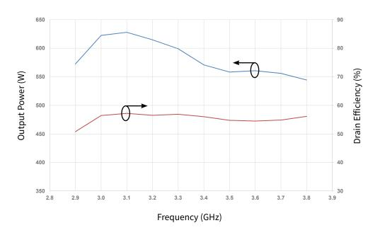
Figure 2. CGHV37400F Output Power and Drain Efficiency vs Frequency  $V_{DD} = 50 \text{ V}, I_{DQ} = 1.0 \text{ A}, P_{IN} = 46 \text{ dBm}, \text{Pulse Width} = 100 \mu \text{s}, \text{Duty Cycle} = 10\%,$  $T_{CASE} = 25^{\circ}\text{C}$
