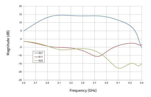
Figure 1. Typical Small Signal Gain and Return Losses vs Frequency  $V_{\text{DD}}$  = 50 V,  $I_{\text{DQ}}$  = 1.0 A
