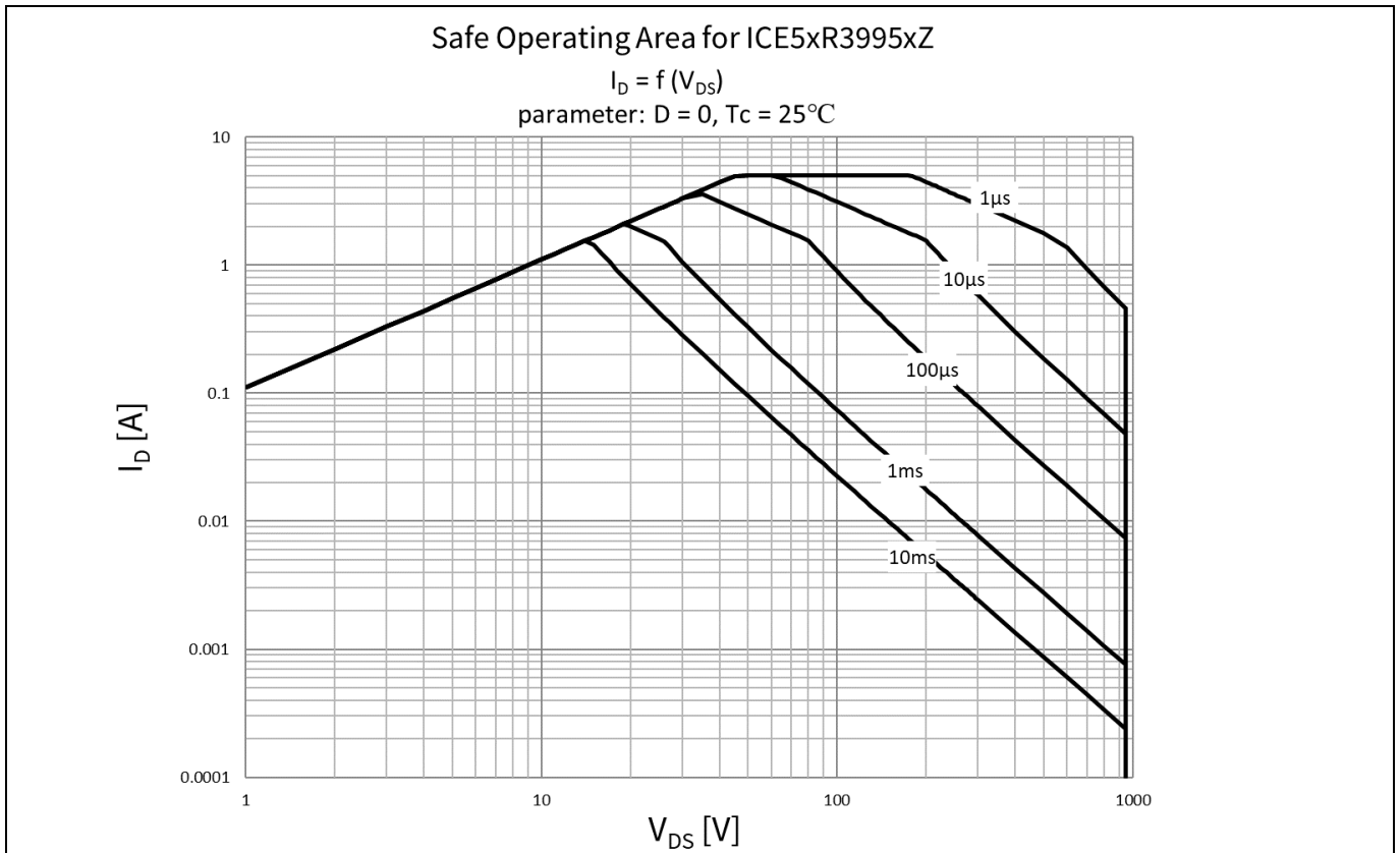
Figure 20 Safe operating area (SOA) curve for ICE5xR3995xZ
