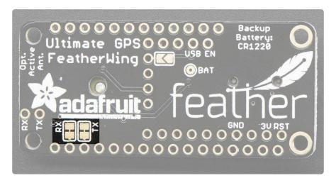
And then wire your desired pins to the RX and TX breakouts right next to the FIX LED
