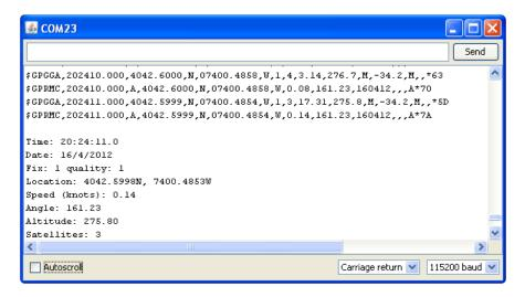
In this sketch, we call GPS.read() constantly in the main loop (if you can, get this to run once a millisecond in an interrupt). Then in the main loop we can ask if a new chunk of data has been received by calling GPS.newNMEAreceived(), if this returns true then we can ask the library to parse that data with GPS.parse(GPS.lastNMEA()).
