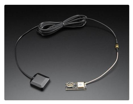
The MTK3339-based module has external antenna functionality. The module has a standard ceramic patch antenna that gives it -165 dB sensitivity, but when you want to have a bigger antenna, you can snap on any 3V active GPS antenna via the uFL connector. The module will automatically detect the active antenna and switch over!
