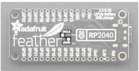
On the back of the board are pads for the SWCLK and SWDIO pins. They provide access to the internal Serial Wire Debug multi-drop bus, which provides debug access to both processors, and can be used to download code.
