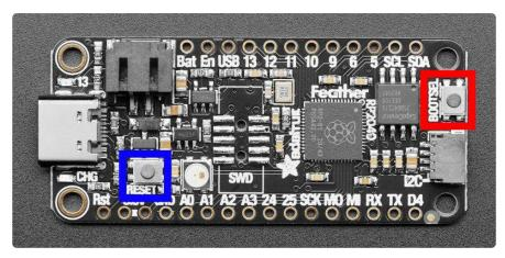
To enter the bootloader, hold down the BOOT/BOOTSEL button (highlighted in red above), and while continuing to hold it (don't let go!), press and release the reset button (highlighted in blue above). Continue to hold the BOOT/BOOTSEL button until the RPI-RP2 drive appears!
