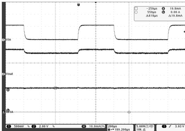
Figure 11. Line Transient Response in 1x Mode, V_{IN} = 3.6\text{ V} - 4.2\text{ V} , I_{LEDx} = 20\text{ mA}
