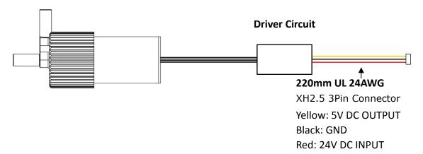
Fig. 1 Wire Schematic
